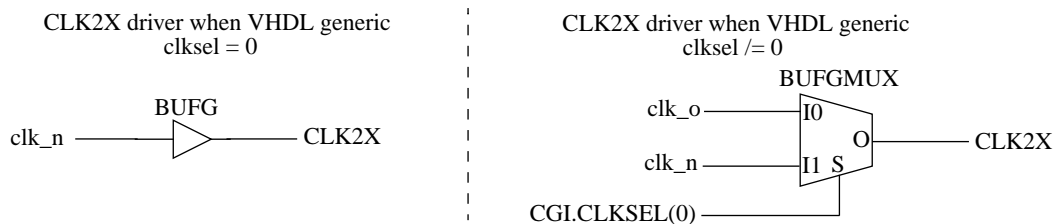
Figure 36. Spartan 3/e selection of CLK2X clock when VHDL generic clk2xen is non-zero
